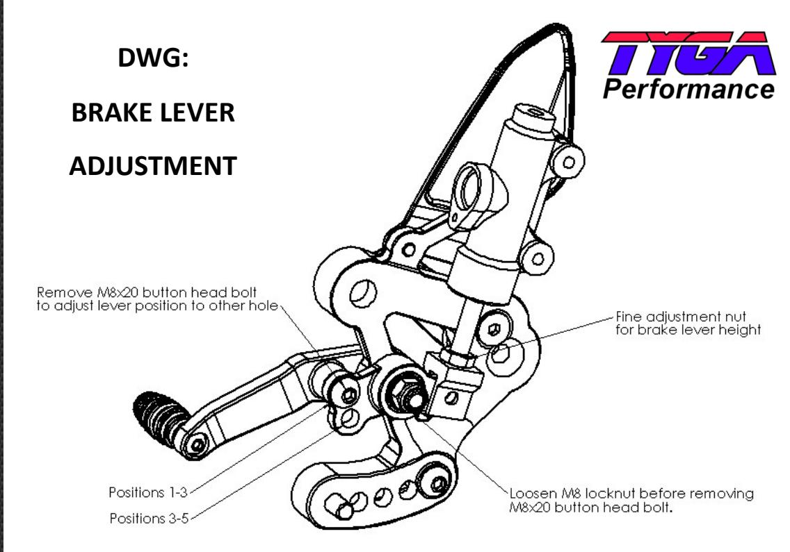
This drawing shows the lever set up for use in position 1-3. To adjust hanger to positions 3-5 the following adjustments are necessary.
