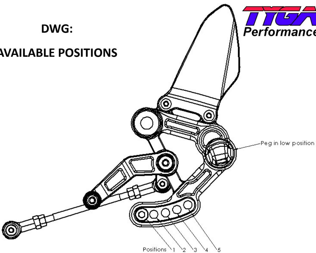
This drawing shows the available positions for the Monkey 125 Step Kit. The left side hanger is shown in the drawing, but the basic adjustment of the hanger is the same for both sides.
