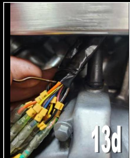
You will notice that wire #4 is not yet connected. This is the 12V for the running lights, so we will connect in a later step. It's advisable to isolate this terminal temporarily to avoid any short circuit during any electrical testing.
