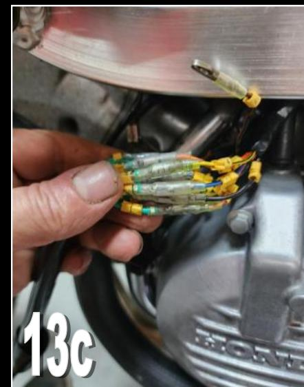
It is a good idea to tape the two sets of wires together as a bit of strain relief
