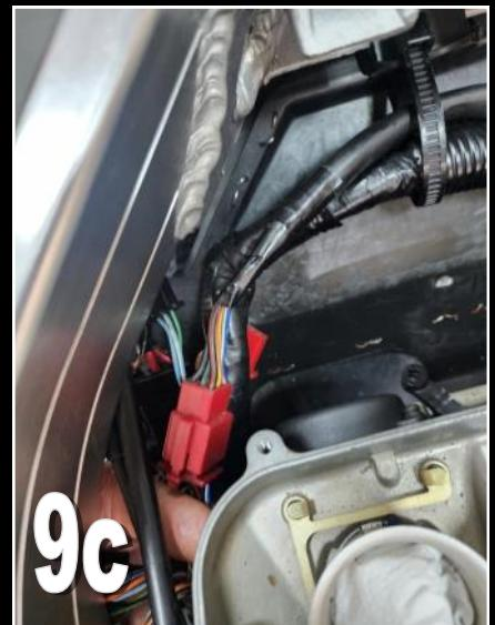
**10)** Now look at the ignition switch wire. For this we need to cut the cable tie that holds the wire to the switch so that we can route it to the left side of the frame and have an adequate length of wire to work with.
