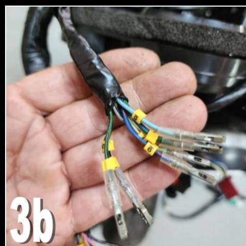
**4)** The exposed terminals from the blue and green 10P connectors will be directly connected to the extension harness that drives the meter and the running lights. This is described later in this document, but we would like to say that we recommend cutting off the original terminals and fitting normal bullet terminals, as the bullet terminals will be 100% compatible with the terminals on the extension harness and will provide a more secure and reliable connection.
