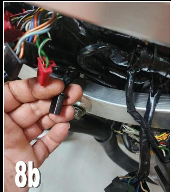
**9)** Moving back to the right hand side of the bike. Route the right hand switch gear wires through the gap between the frame rails and follow the route of the main harness, using the cable tie to secure. Connect the red 9P connector from the switch gear to its mating connectors.
