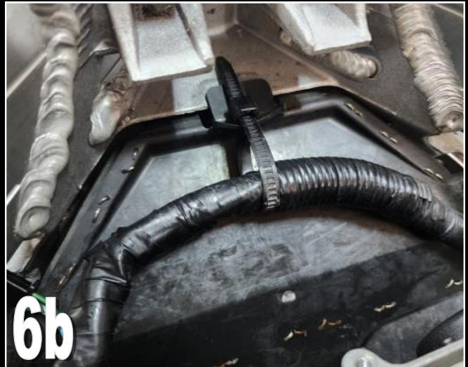
**7)** Now hold the harness as shown, and at an approximate point between the headlight connectors and headlight relay, fold the harness back on itself, and secure the bend with a cable tie.
