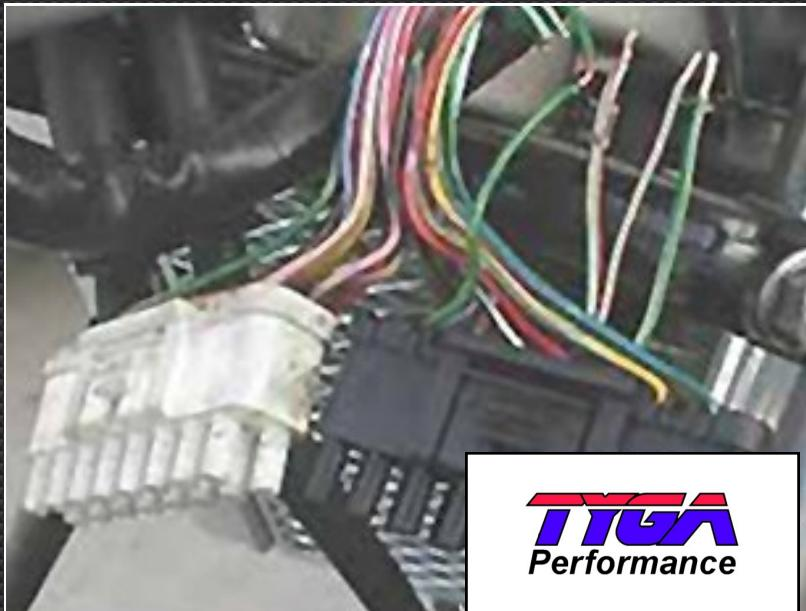
2) Snip the LtGr/R, Gr/P & Gr/W wires approximately 60mm from the black connector, and remove 5mm of insulation to expose the copper wires inside.
